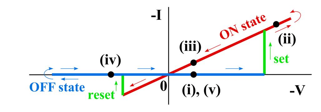
The relationship between the memory effect in an ideal I-V characteristic and measurement points of CAFM for the procedures from (i) to (v).
