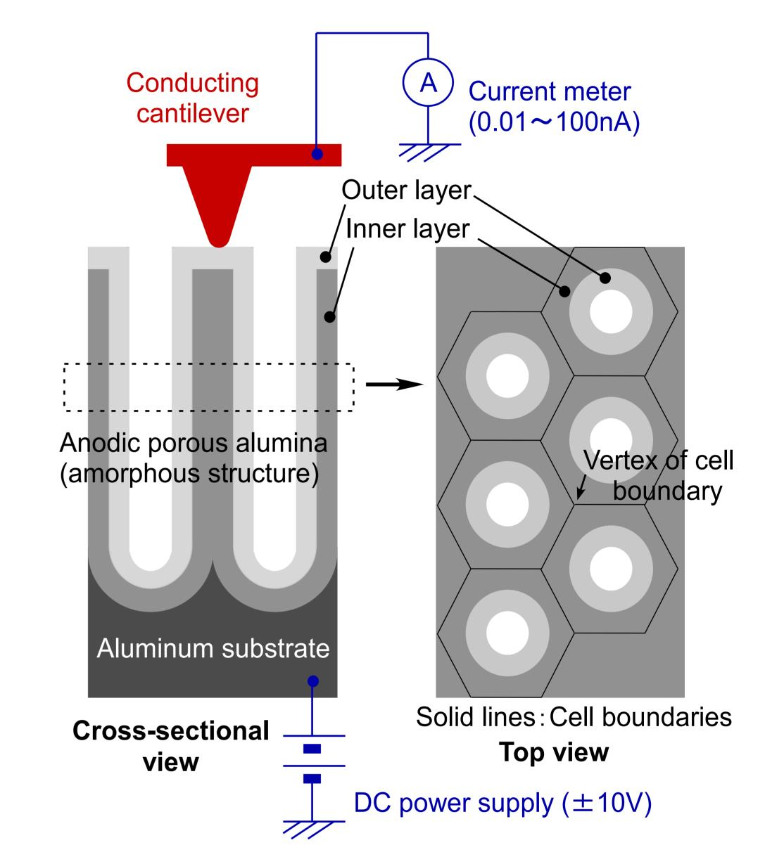
(v) the small negative voltage is applied again to confirm disappearance of the current paths,
